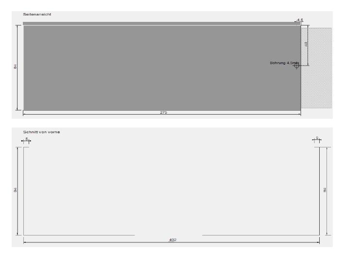
Important when designing your own housing: Ensure good ventilation of the interior parts; connect the metal housing to mains protective earth.
