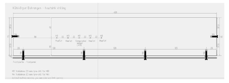
The heat sink is mounted to the front panel using 4 screws type M4 (16 mm length). Use 4 washers per screw so that a vent slot results between the heat sink and the front panel.
