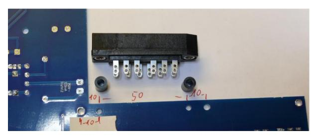
Then connect the female connector to the main board using attenuator pads (VHFchoke + 100 Ohms resistor in parallel) as already depicted. Use heat shrink tube to assure that everything is well insulated. Connect all outward going screws to ground.
