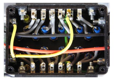
Wiring inside the connector box. The red and black wires are the connection of the measuring device to the circuit board.
