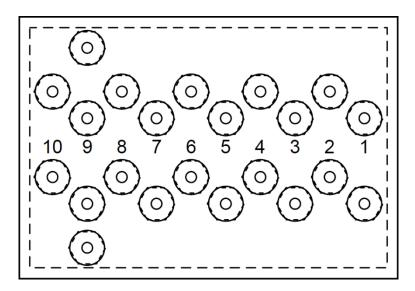
Material used (Reichelt): MBI 1 BLMiniature socket blue20 pieces , 2 mm, MBI 1 GE miniature socket yellow2 pieces , 2 mm, , 72 x 50 x 35 mm1 piece GEH KS 35Small housing Spring-loaded 2mm plug, blue MSTF2 BL asrequired Male connector, 12-pin, DIN 41622, contacts various1 piece ML , 12-pin, DIN 41622, contacts vers. FL B12 female multipoint connector 1 piece
