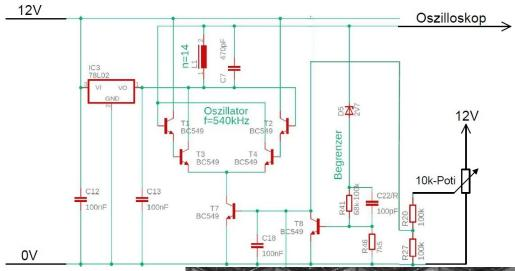
The oscillator output voltage should now be about 700mV rms at maximum control (see the photo at the bottom right of the page). If the oscillator is overdriven (see the photo at the bottom left of this page), the next lower value is set for R41, e.g.  $82k\Omega$ , finer gradations are of course also possible.
