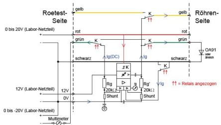
In open circuit, without the OA91 diode, the output voltage rises to over 30V rms. This value is necessary for measuring DK91 tubes with Rg=100k $\Omega$  at 250 $\mu$ A grid current.
