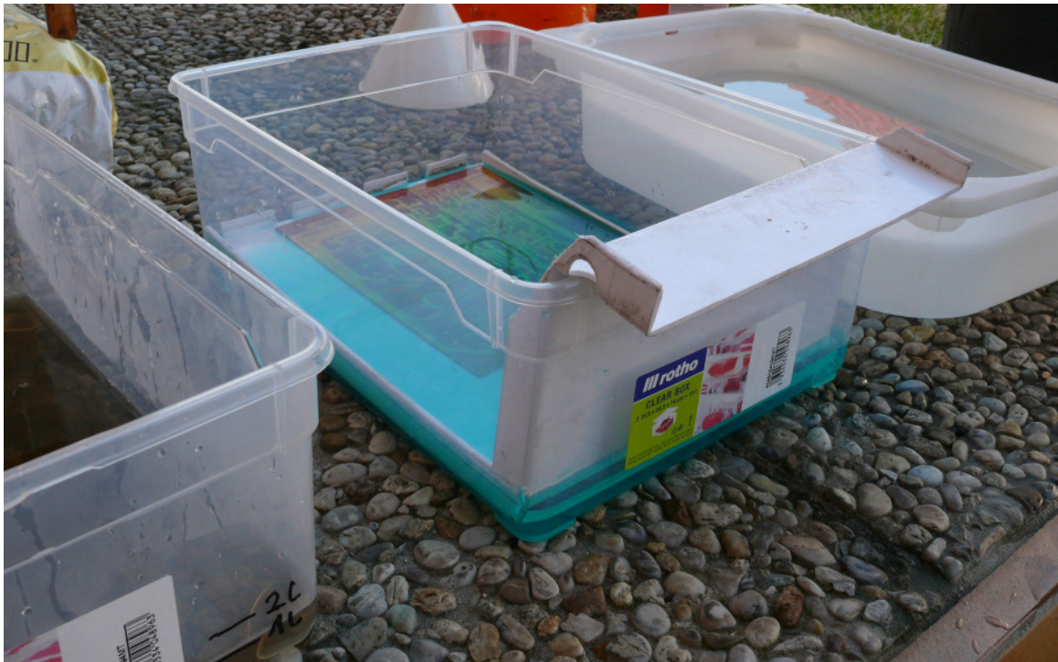
Etching process - Developer, Etching bath and water bath
