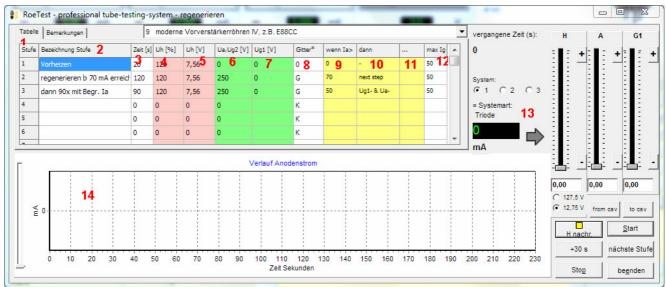
Different modes can be stored in the regeneration database. These modes can be assigned to the specific tubes (tube database) or be selected in the regeneration window (see picture above). In the regeneration window the data may be individually changed (these changes are not permanently stored).
