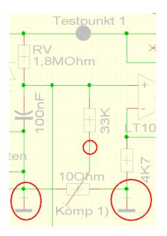
Therefore it's important where the 0 points on the main PCB are connected. Slight voltage variations at the different ground connections impact the amplifier output and result in measurement errors.
