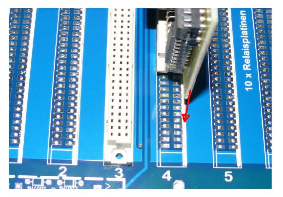
Additional connectors are needed for the A, G2, H and 600V PCBs and you can make these by using a saw to cut up a 64 pin 4mm PCB connector as shown below. You may have to glue the bottom piece back on on the separated pieces:
