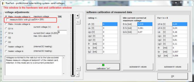
Set the anode board output to 280V and then calibrate the G3 board by adjusting the trim pot for the 600V range on the G3 board until it indicates 280V. Note: you can only do this if you have set the correct version of the G3 card in the software (Options/test->Options) and your G3 card must be version 6 or higher. Otherwise the checkbox will not be displayed on the screen. Never connect the cards using a wire!
