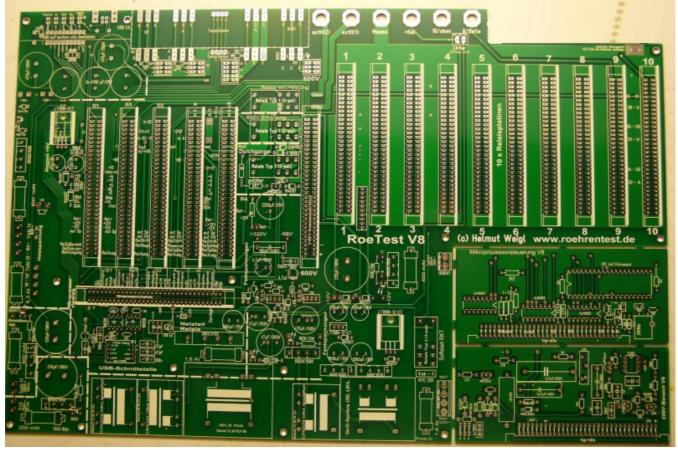
Voltage PCBs: despite single sided layouts no wire bridges are needed. You can separate the PCBs for instance by bending them on a table edge right at the PCB edges.
