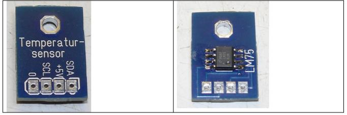
This PCB must be mounted to the heat sink in such a way that the LM75 IC touches it. I recommend the use of thermal compound between the IC and the heat sink. Be sure to insulate the pins to heat sink.
