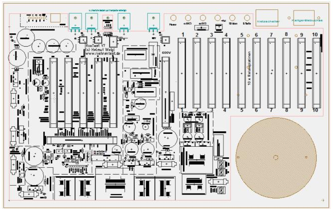
Front panel seen from behind with main PCB and the spot for the toroid transformer. The sockets for the required connections (USB, banana sockets, mains switch etc.) are on the front side. You can also see the locations of the MOSFETs and the temperature sensor Mounting of mainboard on the front panel for a RoeTest V7 – this shows the way the V8 motherboard would look after cutting along the dashed lines where the MOSFETs are connected.
