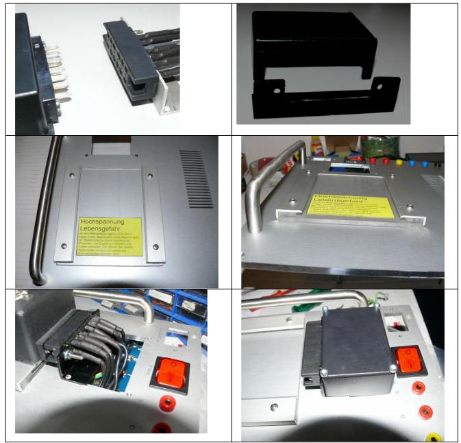
The socket box receiver is made from plastic (clear acrylic or similar) and an aluminum angle and has two rails to guide the socket boxes. Make sure that the bolts are not too long and touch the PCB or the main transformer. Make sure to bolt the main transformer to the frontpanel before bolting on the socket box receiver.
