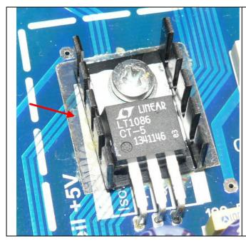
The heat sink for the 5V voltage regulator must be **insulated** from the main PCB to avoid a short circuit between the heat sink and the traces underneath it. I have used a tranparent plastic sheet and glued it between the traces and the heat sink as shown here.
