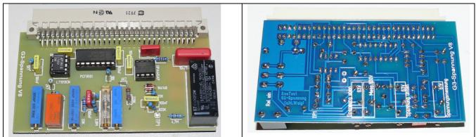
The G3 PCB from version 6 onwards has an additional function: if the board is not used to generate a G3 voltage it can be used to measure voltages up to 600V. For that purpose the PCB has an additional trimmer resistor for calibration purposes. This funkction is used at testing voltage stabilizers.
