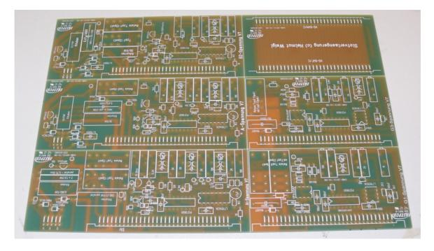
And finally the relay matrix PCBs. Also here despite single sided layouts no wire bridges are needed. You can separate the PCBs for instance by bending them on a table edge right at the PCB edges.
