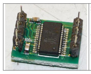
Adapter board seen from the bottom. Here you can see the two SMD capacitors (100nF, type 805).
