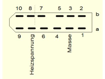
Connection diagram for the DIN 41622 connector (seen from front on socket box receiver)
