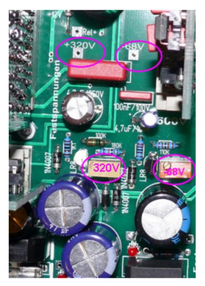
Variable/microcontroller controlled output voltages:
