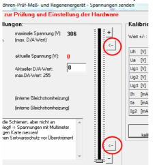
Adjust the trim pot marked "unten, kleiner Bereich" on the anode PCB until your multimeter indicates the same voltage as the value shown in red on the screen.
