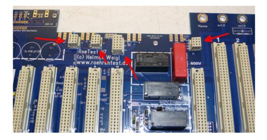
Picture of the V7 main PCB: an industrially made PCB has many advantages over home made PCBs: silk screening, solder mask, double sided with vias, exact fit...all this just saves many hours of work, making it a good investment.
