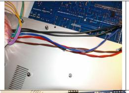
Main transformer connections to main PCB: route the wires in between the PCB and the front panel. You may want to twist the wires together, as this will help to suppress mains supply and RF frequency interference.
