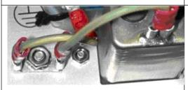
Connect ground wire coming from the mains to front panel, case and PCB with wires. This way all metal parts that can be touched from the outside are grounded.
