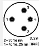
The numbering of the sockets can be seen in the socket database. The following applies: Always the tube seen from below (also for german WWII tubes)
