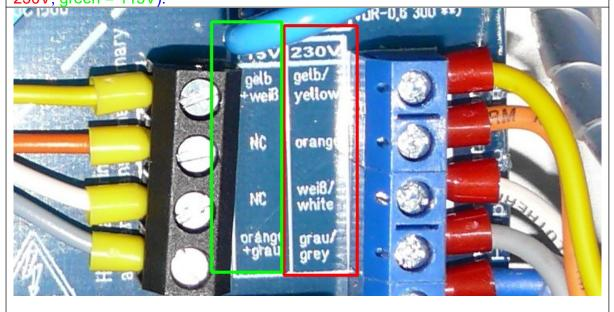
This picture is showing the connection of the both transformers at 230V mains voltage.
