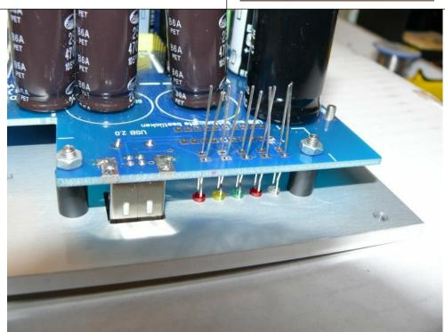
The LEDs are soldered in after the PCB is attached to the front panel so that it's easy to solder them in at the correct height. When installing the LEDs, the longest wire is the anode.
