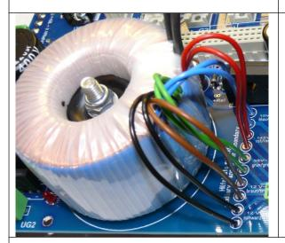
Secondary connections, the circuit board is labeled with the cable colors
