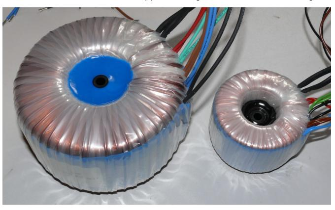
Main transformer and auxiliary transformer (made to specification, avialable from me)
