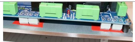
To avoid short circuits or flash overs I used duct tape between the connectors and the front panel (red)
