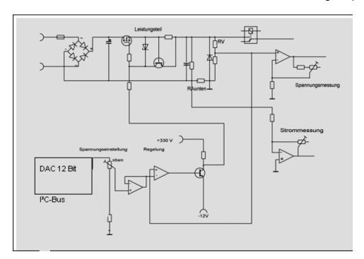
A D/A converter that is connected to the I²C-Bus is controlled by the PIC and generates a 0 to 4,7V voltage and that voltage is amplified using an opamp and a transistor. The H, A and G2 circuits use MOSFETs for increased power output.
