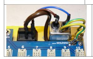
There is a 6,3mm flat connector for connecting the protective earth to the mainboard.
