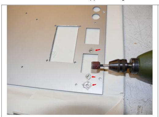
Grounding: All screws must have good electrical contact with the front panel. For this purpose, the anodized layer on the back must be sanded off at the marked points.
