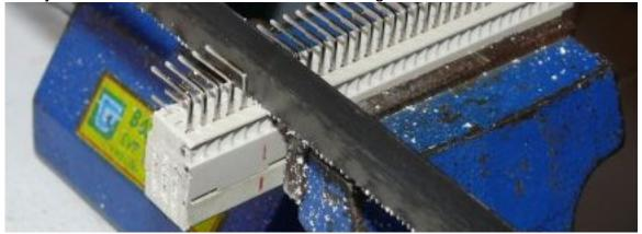
remove the pins at the cutting position before cut
