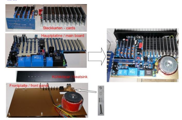
Info: The above pictures shows still the old main transformer. The new transformer needs no rubber and no metallic disc.
