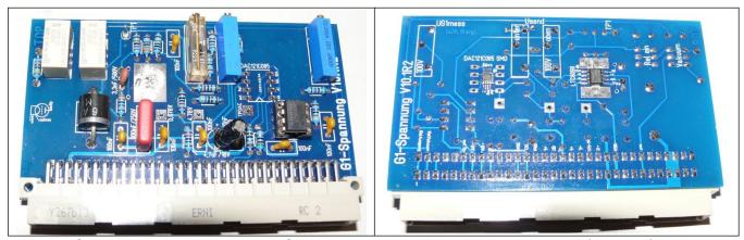
The LTC6090 is soldered on the PCB's bottom side. There is an exposed (thermal) pad on the bottom side of this IC that also must be soldered to the PCB (see hint: "Don't be afraid of SMD components"). This also applies for the G3 board.
