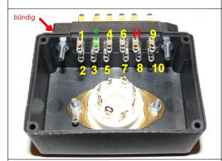
Numbering of the pins at rotated adapter box.
