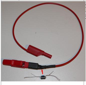
Jse an insulated alligator clip. An attenuator nust be installed directly on the terminal VHF choke, parallel to a resistor of 100 Dhm, 0.6W, metal film)
