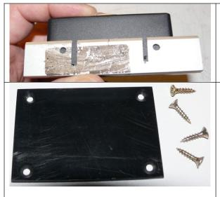
Drilling template: This can be made from a piece of aluminum angle and provides a guide for drilling and cutting.
