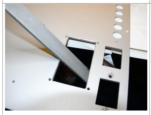
The back of the opening for the socket box connection should be rounded off slightly with the file so that the cables do not chafe through.
