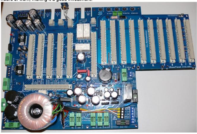
Top side of main PCB this allows alternatively mains voltages of 115V (110-120V) or 230V (220-240V) 50/60Hz.
