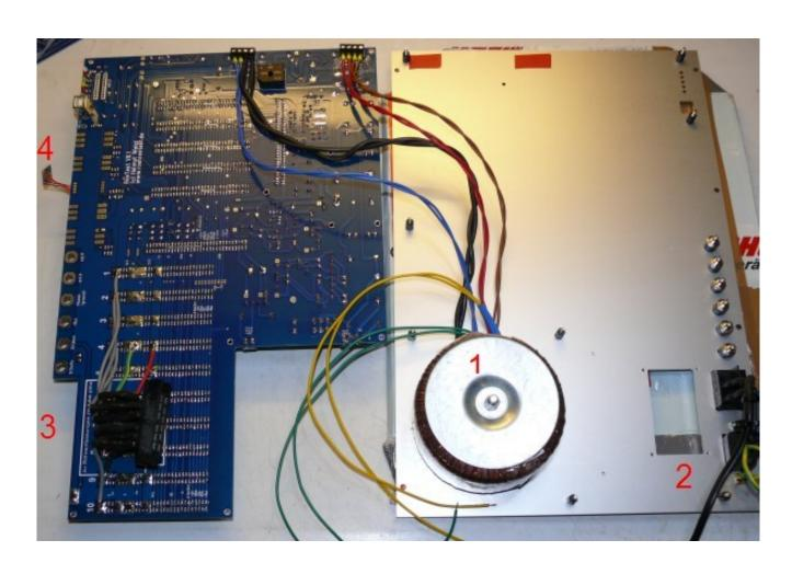
Important: keep all wires to the socket box receiver and to the MOSFETs as short as possible. The longer the wires, the more risk there is for oscillations with certain tube types.
