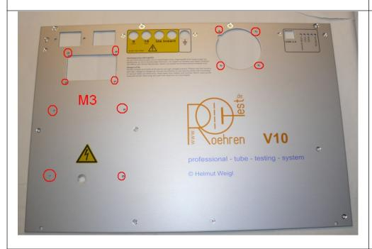
The anodizing also has to be removed from the M3 threaded holes so that the screws have electrical contact with the front plate (earth).
