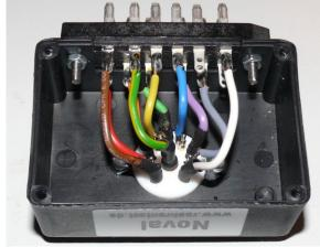
Make sure to connect any metal parts that can be touched to ground. Also screws. It is easier using plastic screws.
