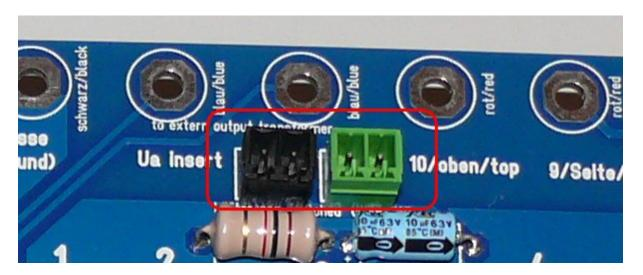
Picture of the main PCB: an industrially made PCB has many advantages over home made PCBs: silk screening, solder mask, double sided with vias, exact fit...all this just saves many hours of work, making it a good investment.
