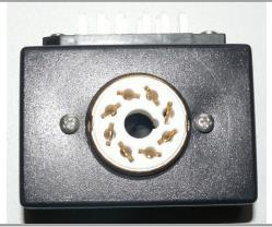
It's best to have only one tube socket per socket box. That way wiring can be kept simple and there is less chance for oscillations.
