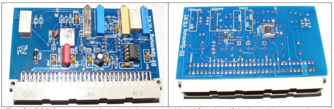
The G3 PCB from version 6 onwards has an additional function: if the board is not used to generate a G3 voltage it can be used to measure voltages up to 600V. For that purpose the PCB has an additional trimmer resistor for calibration purposes. This function is used for testing voltage stabilizer tubes.
