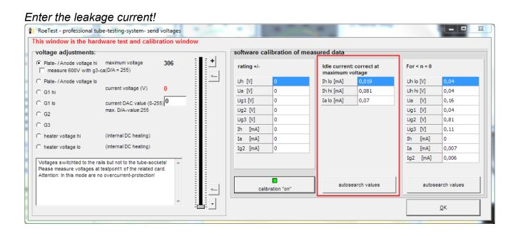
If the meters don't read zero at idle condition, the settings in the right column can be used.
