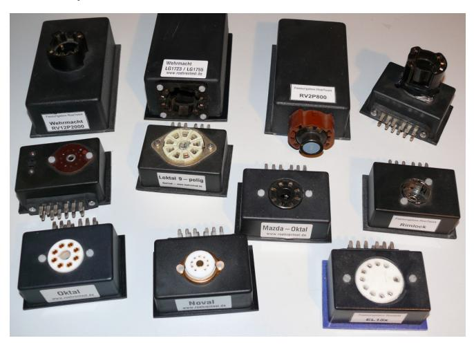
Here are some examples of the tube socket boxes I'm using. The low cost plastic boxes get new bottom plates that are wider than the box itself (in my case it's 80 mm wide) so they fit into the rails of the socket box receiver.
