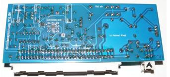
Please solder on the bottom site of the PCB the DAC121C085 and a USBLC6-2SC
