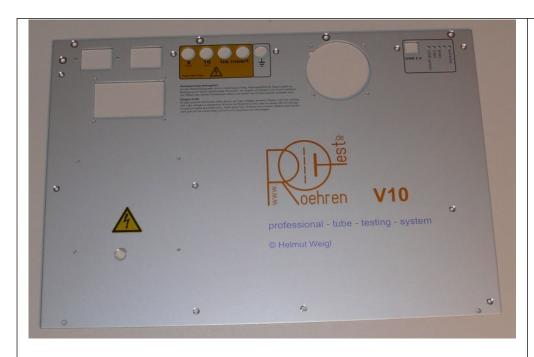
Front panel (V10) professional quality, manufactured according to my specifications by a leading German manufacturer, 3 mm aluminum, under anodized print (smudge-proof and scratch-proof, oil- and thinnerresistant), also anodized edges, cutouts and drill holes perfectly fitting
