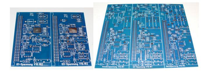
And finally the 10 relay matrix PCBs. You can separate the PCBs for instance by bending them on a table edge right at the PCB edges.
