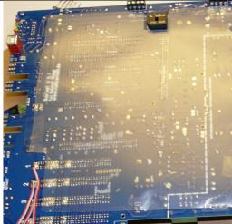
In order to protect the wires between main board and frontpanel, please glue a plastic film on the bottom site of the mainboard (with tape)
