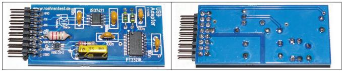
The USB interface is located on a **separate board that is plugged onto the mainboard**. USB female jack and the LEDs are located at the upper left edge of the mainboard.
