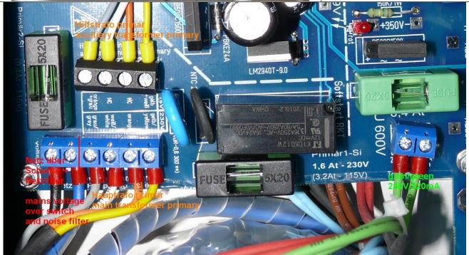
The mainboard connectors close to the toroid transformer are mounted on the top side of the PCB. The cable for the mains connection is also routed in between the front panel and the PCB. I used regular 2 wire mains cable.
