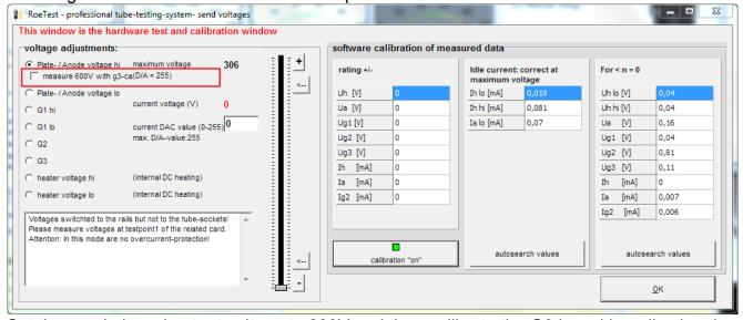
Set the anode board output voltage to 280V and then calibrate the G3 board by adjusting the trim pot for the 600V range on the G3 board until it indicates 280V. **Note: you can only do this if you have set the correct version of the G3 card in the software (Options/test->Options) and your G3 card must be version 6 or higher.** Otherwise the check-box will not be displayed on the screen. **Never try to connect the cards using a wire!**
