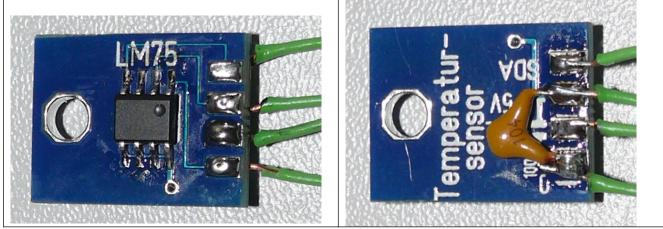
This PCB must be mounted to the heat sink in such a way that the LM75 IC's upper side touches the heat sink. I recommend the use of thermal compound between the IC and the heat sink. Be sure to insulate the pins from the heat sink.
