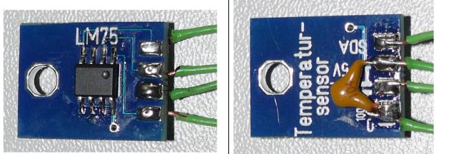
This PCB must be mounted to the heat sink in such a way that the LM75 IC's upper side touches the heat sink. I recommend the use of thermal compound between the IC and the heat sink. Be sure to insulate the pins from the heat sink.
