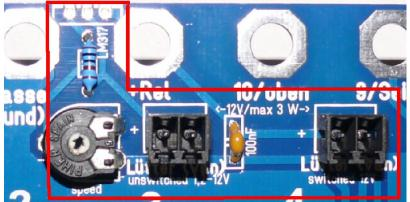
These components need only be mounted when a fan/fans is/are used.
