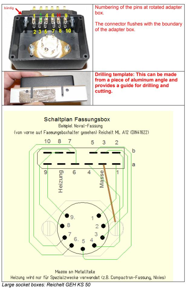
Small socket boxes: Reichelt GEH KS 35 Male connector (DIN41622): Reichelt ML A12 For tubes which are very prone to oscillation:
