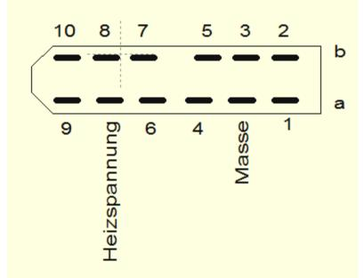
Connection diagram for the DIN 41622 connector (seen from the front on the socket box receiver)
