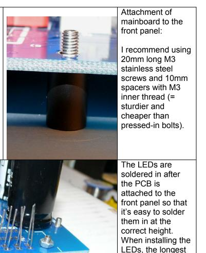
Mount USB jack and LEDs on mainpanel's bottom side!
