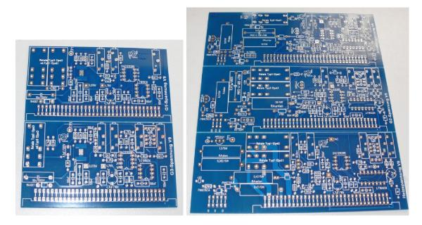
And finally the 10 relay matrix PCBs. You can separate the PCBs for instance by bending them on a table edge right at the PCB edges.
