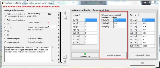
If the meters don't read zero at idle condition, the settings in the right column can be used. Do this with the button <autosearch values> with RoeTest connected
