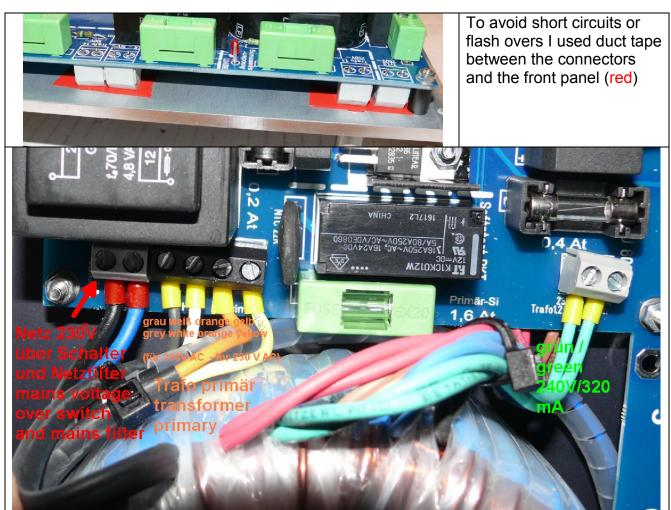
The mainboard connectors close to the toroid transformer are mounted on the top side of the PCB. The cable for the mains connection is also routed in between the front panel and the PCB. I used regular 2 wire mains cable.
