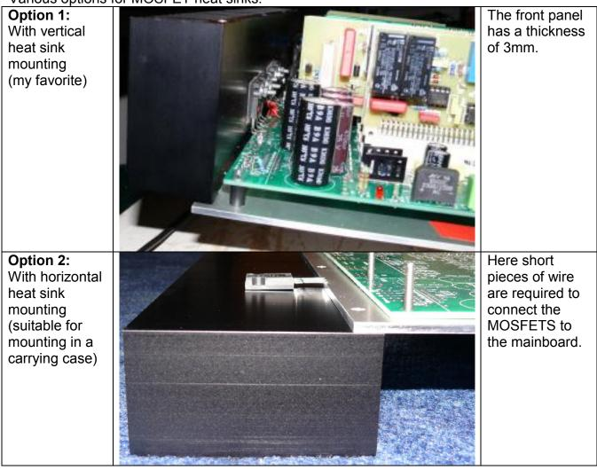
The MOSFETs must be insulated from the front panel or heat sink. I suggest Kapton insulation with only 0.15 K / W thermal resistance. Insulation with poorer properties should be avoided because the MOSFETs could overheat before the heat is passed to the heat sink. The MOSFET connectors are soldered directly to the motherboard.
