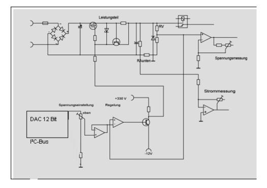
A D/A converter that is connected to the I<sup>2</sup>C-Bus is controlled by the PIC and generates a 0 to 4,7V voltage and that voltage is amplified using an opamp and a transistor. The H, A and G2 circuits use MOSFETs for increased power output.
