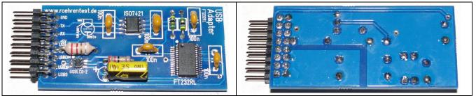
The USB interface is located on a **separate board that is plugged onto the mainboard**. USB female jack and the LEDs are located at the upper left edge of the mainboard.
