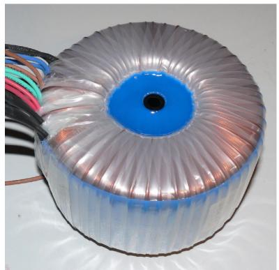
Main transformer = toroid transformer (made to specification)
