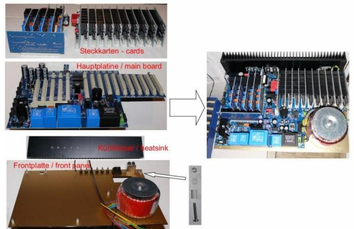
The front panel with all electronics bolted to it can be put in an aluminum suitcase or some other suitable cabinet.
