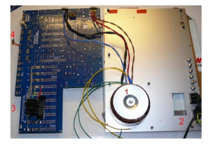
**Important: keep all wires to the socket box receiver and to the MOSFETs as short as possible.** The longer the wires, the more risk there is for oscillations with certain tube types.
