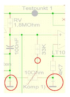
Therefore it's important where the GND points on the main PCB are connected. Slight voltage variations at the different ground connections impact the amplifier output and result in measurement errors.
