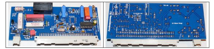
Please solder on the bottom site of the PCB the DAC121C085 and a USBLC6-2SC
