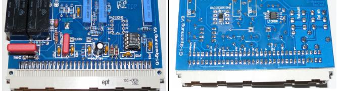
The LTC6090 is soldered on the PCB's bottom side. There is an exposed (thermal) pad on the bottom side of this IC that also must be soldered to the PCB (see hint: "Don't be afraid of SMD components"). This also applies for the G3 board.
