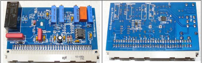
The G3 PCB from version 6 onwards has an additional function: if the board is not used to generate a G3 voltage it can be used to measure voltages up to 600V. For that purpose the PCB has an additional trimmer resistor for calibration purposes. This function is used for testing voltage stabilizer tubes.
