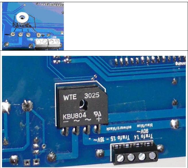
The 10 mm spacer is shown for comparison. At this location you don't need to use a spacer since the plastic washers and the bridge rectifier are effectively used as a 10 mm spacer here.
